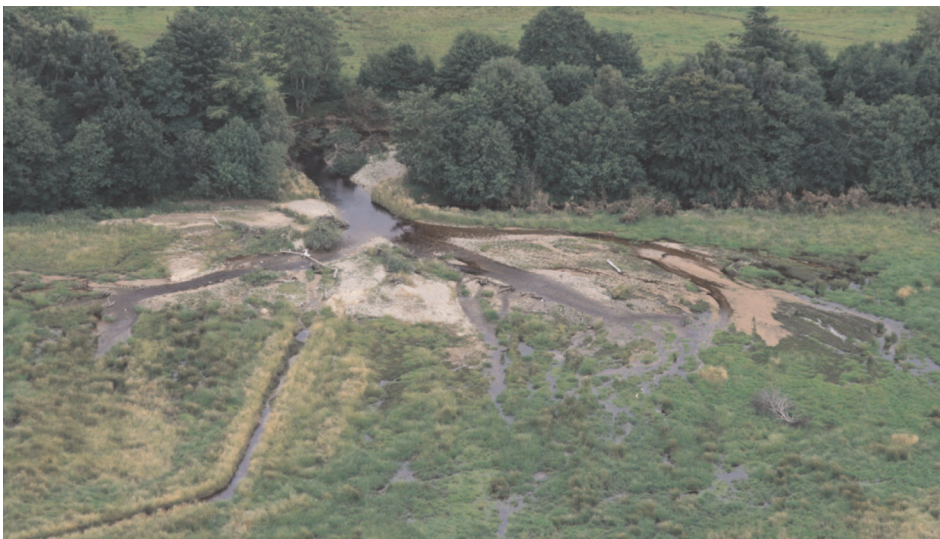
Figure 14.8 Anabranching downstream of the upstream breach following the 4 September 2009 flood event. Note the development of anabranching upstream of the straight, pilot channel in the left foreground
