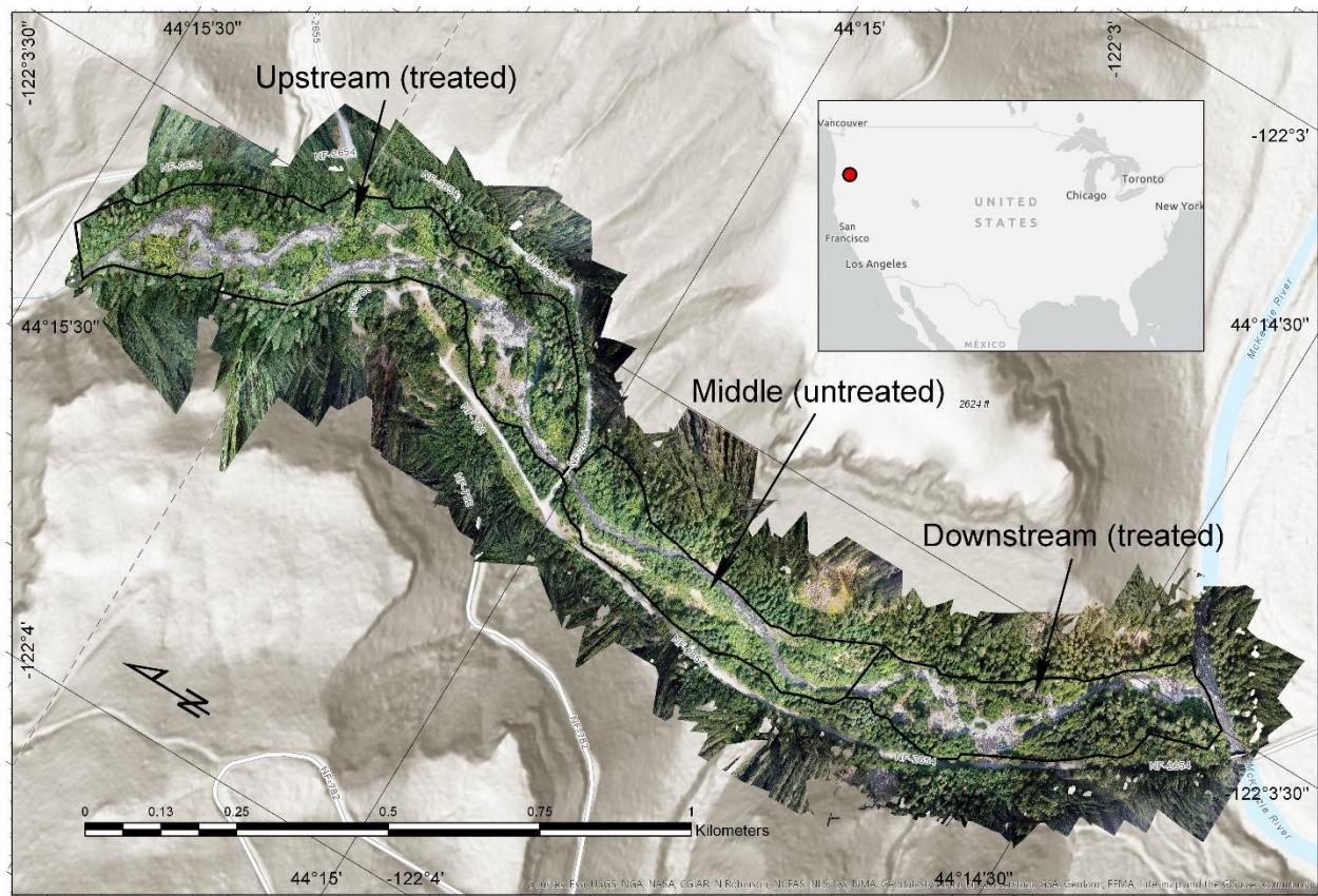
Figure 2: Map showing the three reaches of the Deer Creek Stage 0 restoration project overlaid on a drone-derived orthomosaic from August 2018. Inset shows Deer Creek (red circle) location. Black boundaries delineate the valley bottom extent mapped for each reach.
